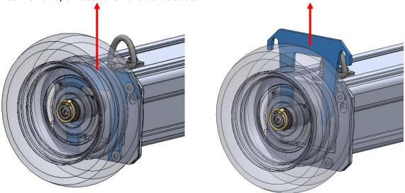
Walk back around to the side where the handle is and remove the 3/16" lynch pin and retainer that holds the bump wheels on, before removing the entire wheel assembly.
