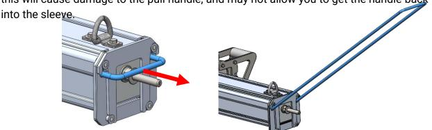
Grip the stainless-steel pull handle firmly and pull towards you. In the case where there is lots of debris collected, you may need to first pull swiftly to get the sleeve started off the magnet housing. It should get easier the further you pull the sleeve off.
