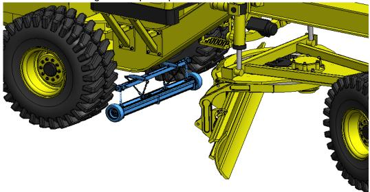
Note: The bump wheels on the ends of the sweeper should no less than 1/2"-1" off the ground when on level ground. The bump wheels on the sweeper will help to prevent ground strikes to the magnet housing and quick clean off sleeve. If you notice that the wheels on the ends of the sweeper are rolling on the ground frequently, it is recommended to raise the sweeper to prevent damage to the aluminum quick clean off sleeve.
