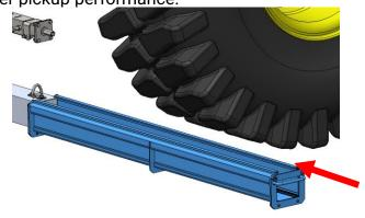
The debris that was collected will be piled up on the ground on one end of the sweeper. Sweep up this debris and place it in a designated scrap or garbage bin. Alternatively, you can use a Bluestreak Powerstik to easily pickup and discard debris. Always wear gloves when handling metal debris to avoid cuts or other injuries.
